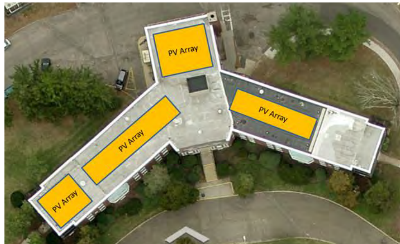
Figure 13: Roof of Ammerman Building with possible PV array arrangement.
