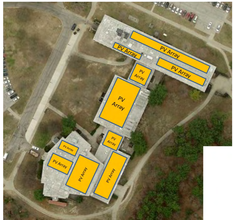
Figure 11: Roof of Islip Arts/ Shea Theater with possible PV array arrangement.
