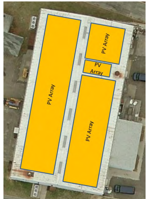
Figure 29: Roof of Trade Shop with possible PV array arrangement.
