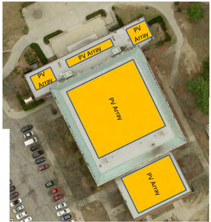
Figure 12: Roof of Brookhaven Gym with possible PV array arrangement.
