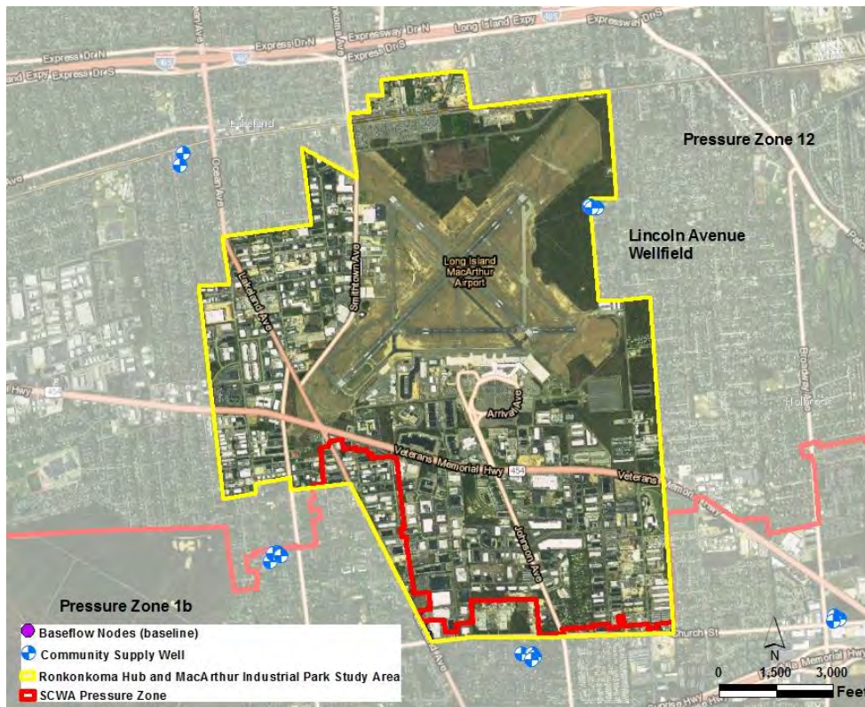
Figure 2 SCWA Pressure Zones and Wells Surrounding the Ronkonkoma Hub/MacArthur Industrial Park Study Area
